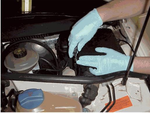
Loosen and remove the five 8mm screws attaching the Engine Control Module top cover to the case assembly. This is located in the rearmost section of the engine bay on the driver's side of the car.
